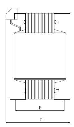
Technical data: Input 230.V at 50/60 Hz and Output 400.V
